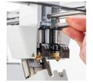
Print cores AA and BB Quick-swap nozzles for build and water-soluble support materials
